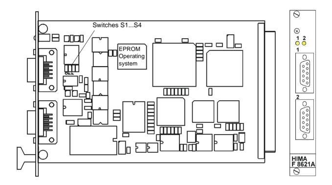
The coprocessor module has its own microprocessor HD 64180 and operates with a clock frequency of 10 MHz. It contains mainly the following functions:
