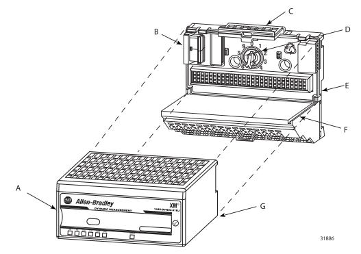
2. Make sure the side connector (B) is pushed fully to the left.
